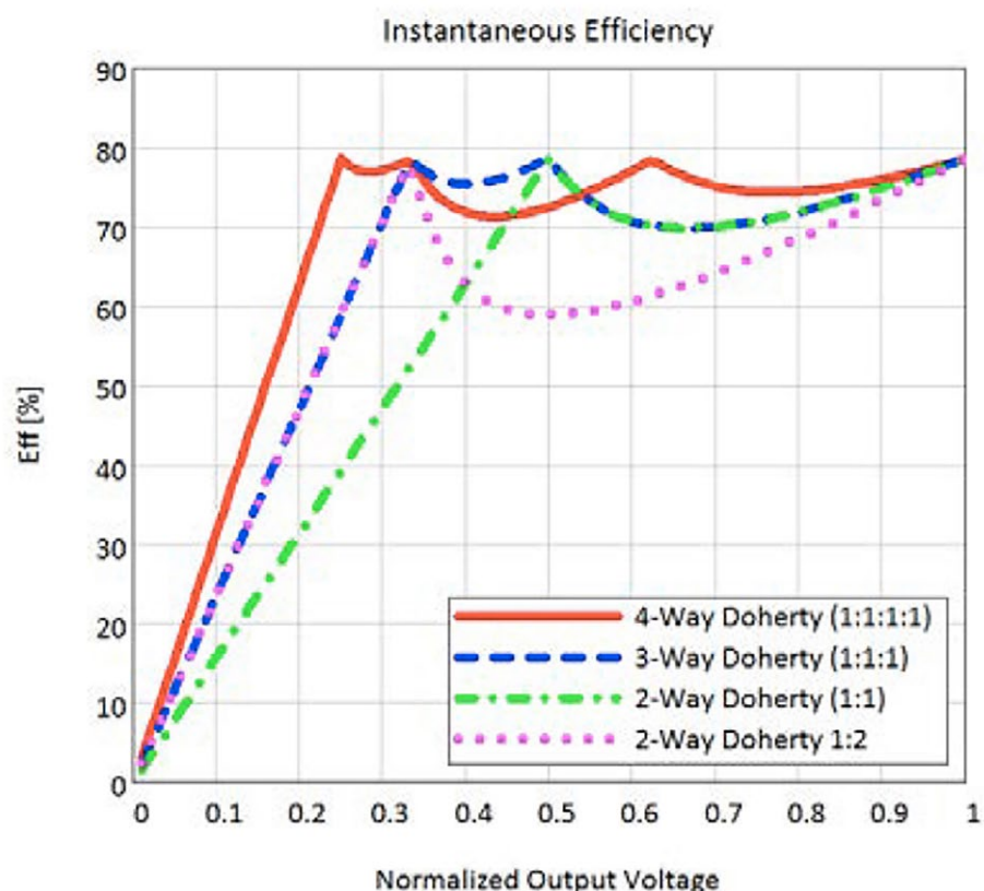
Figure 2: Comparing the efficiency of various DPA architectures (Source: Ampleon).
