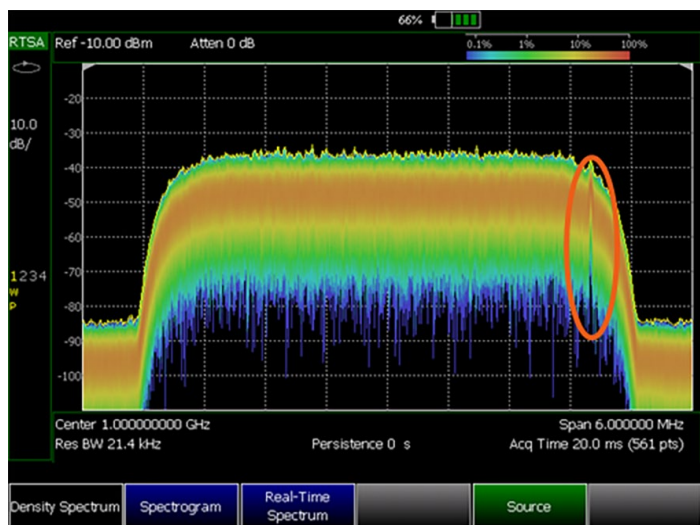
Figure 3: This measurement reveals a suspicious narrowband RF signal trying to hide beneath a W-CDMA carrier signal.
